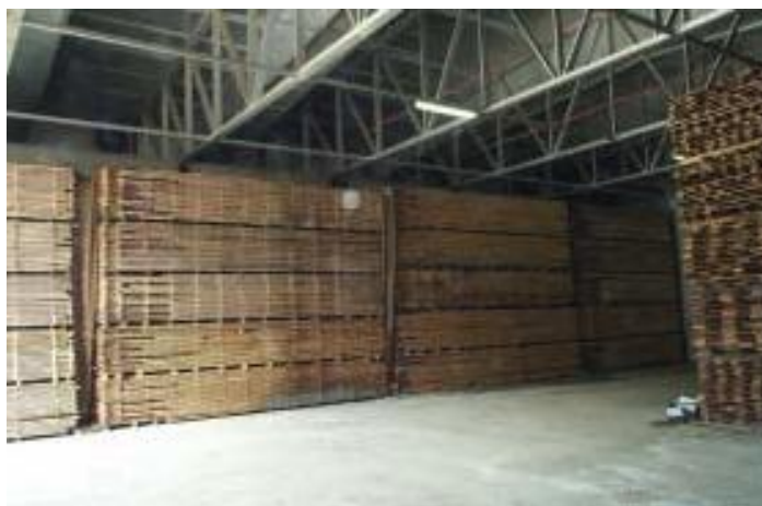
Figure 9.19. Same length racks in a predryer
