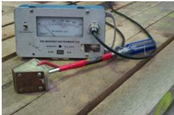
Figure 16.12 Resistance meter with nail connector
