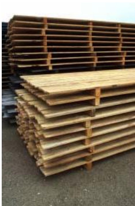
Figure 8.26 Simple pallet style rack covers made from low grade boards
