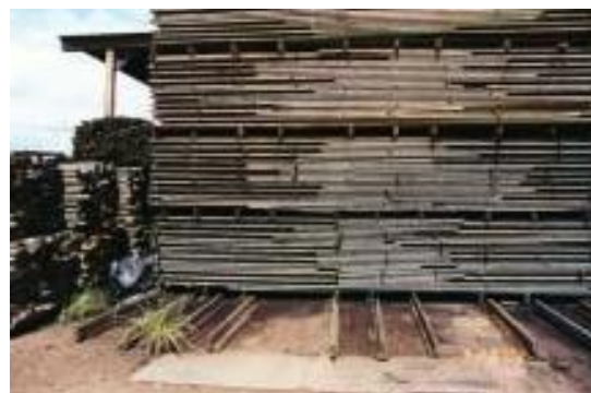
Figure 8.31 Undesirable - Not repeating the position of bearers and gluts under the upper ones
