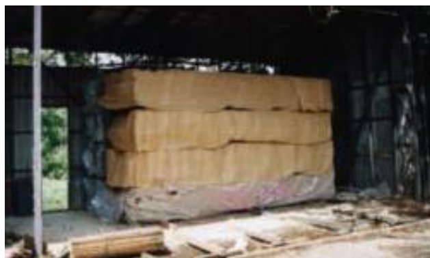
Figure 8.08. Wrapped stack in a shed during initial drying
