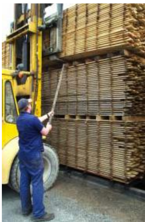
Figure 8.32. Aligning bearers and gluts
