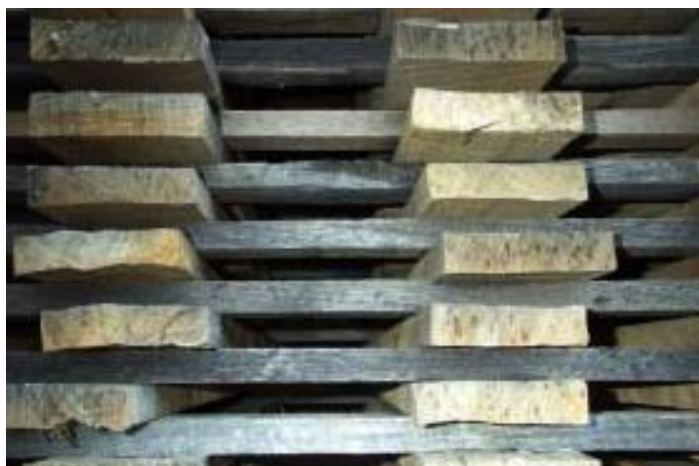
Figure 10.02. Collapse in boards before reconditioning
