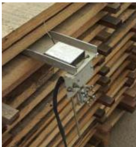
Figure 9.17: An EMC wafer used in a predryer
