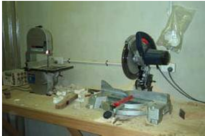
Figure 16.14. Preparation station with docking and band saws for cutting test samples
