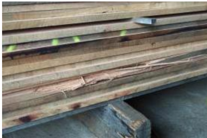
Figure 12.13. Forklift damage to a KD pack
