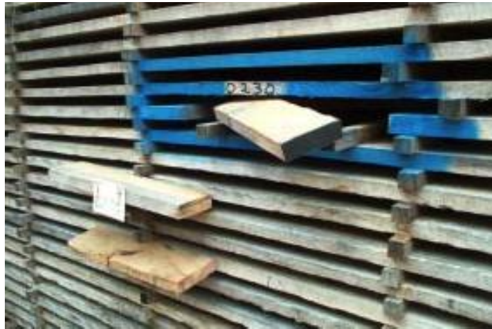
Figure 16.06. Sample board with two outside cover boards
