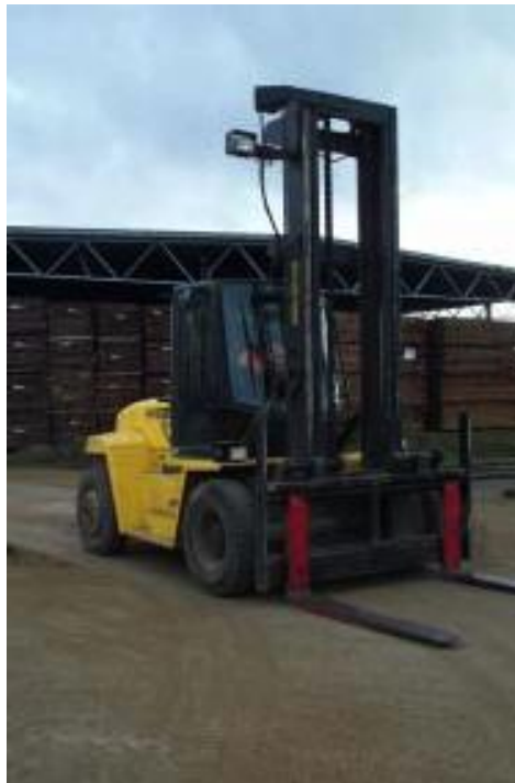
Figure 8.25. Fork lift rated for 12 tonnes
