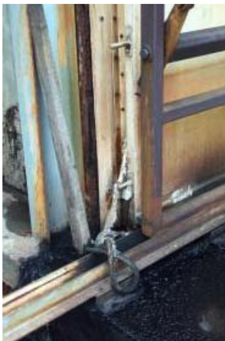
Figure 10.06 Broken door seal releases steam
