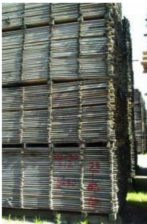
Figure 8.47. Missing bearers cause board distortion
