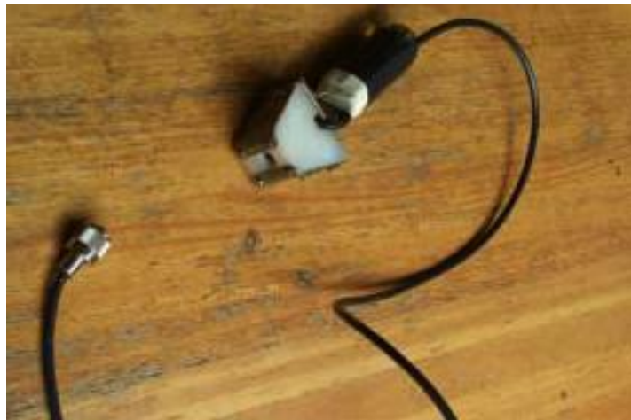
Figure 16.03. Nail (pin) contactor for a resistance meter
