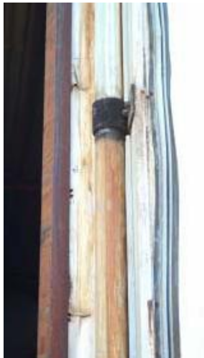
Figure 11.11. Kilns seals need to be inspected regularly and repaired as required
