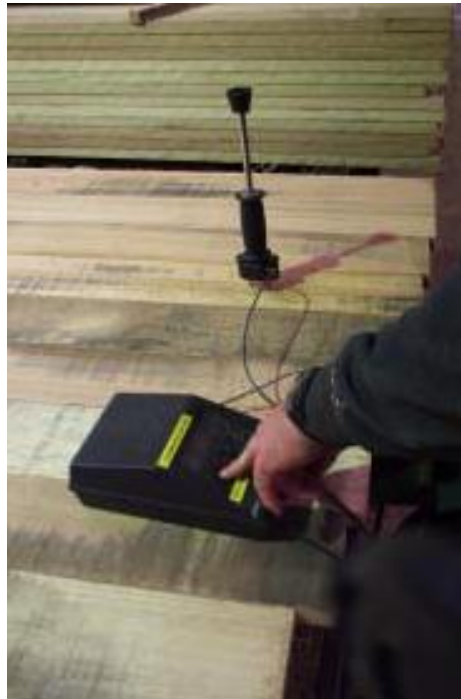
Figure 12.02. Checking moisture with a resistance meter
