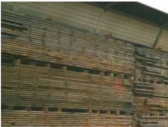
Figure 11.12. Desirable: Baffles correctly placed
