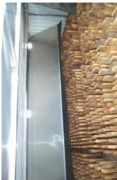
Figure 9.02. A hinged solid baffle with a flexible edge in position in a predryer. Square ended racks are essential for effective baffling
