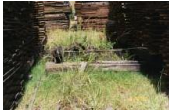
Figure 8.36. Undesirable: weeds under stacks
