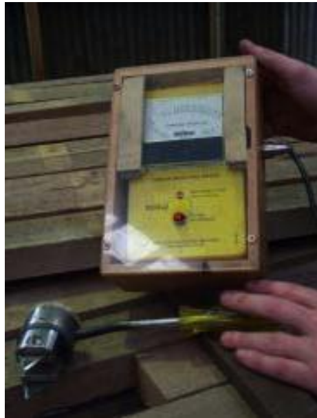
Figure 16.11 Resistance meter with blade electrodes
