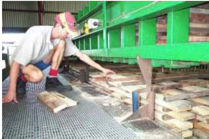
Figure 16.07. Building a test sample into the rack as it is assembled
