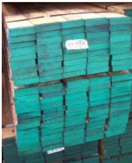
Figure 5.10. Pack number on end coated packs
