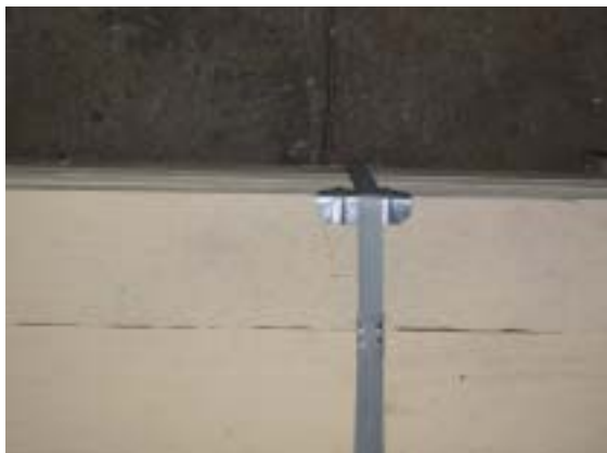
Figure 5.06. Desirable: Corners protected from pack straps
