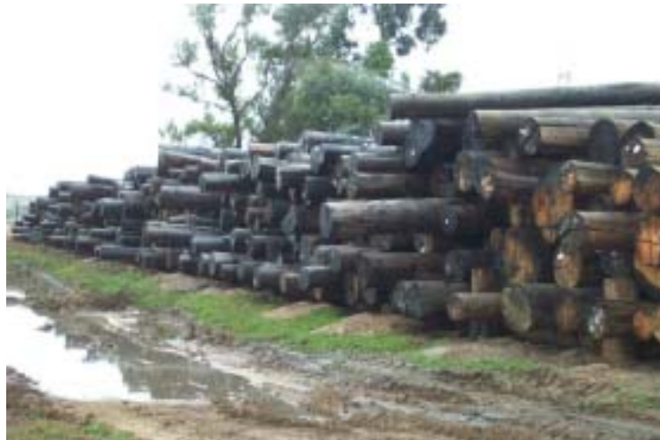
Figure 3.12. Mud associated with poor drainage in a sprinkled log yard
