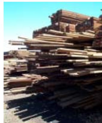
Figure 5.03. Undesirable: Pack with uneven ends
