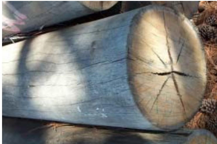
Figure 2.02. End and barrel checking of unprotected logs
