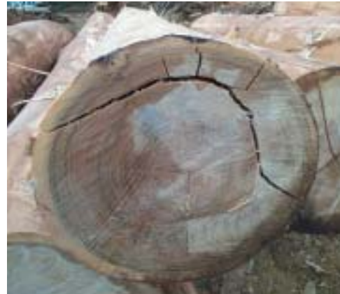
Figure 2.04. Log end splitting, caused by felling, initial drying, growth stress release or all three
