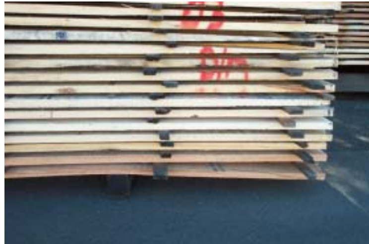
Figure7.39. Bearer poorly placed
