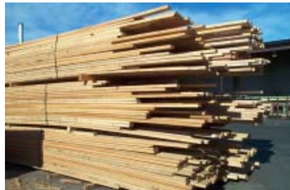
Figure 5.12. Undesirable: Uneven sides and ends
