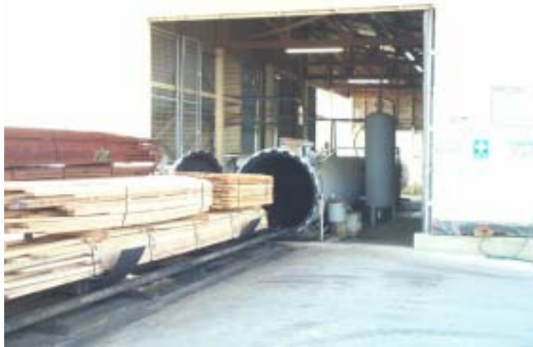
Figure 6.02 Chemical treatment pressure cylinder
