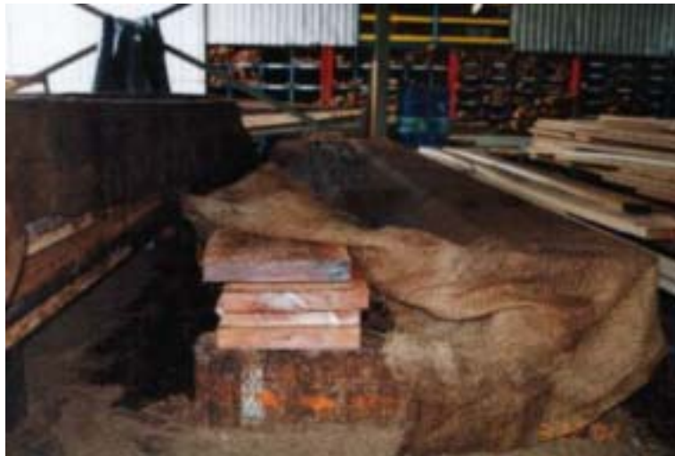
Figure 4.15. Protected Boards stacked under shelter
