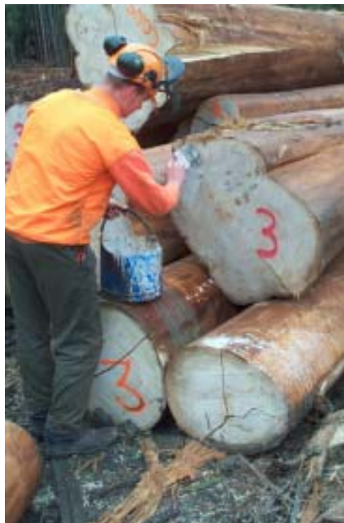
Figure 2.03 End sealing logs as they are graded
