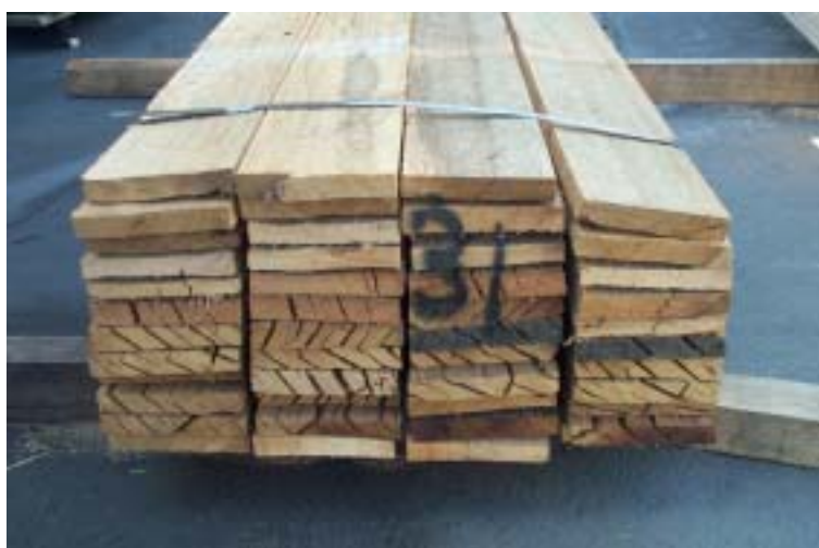
Figure 5.09. End checking from exposure during transport
