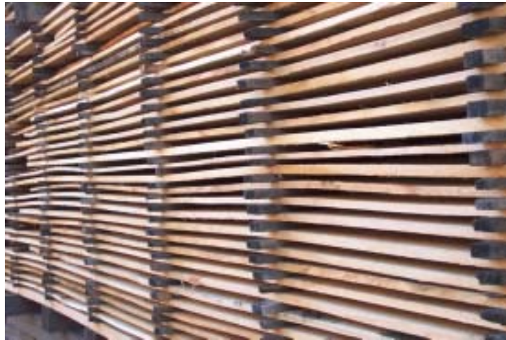
Figure 7.02 Inadequate rack stick spacing
