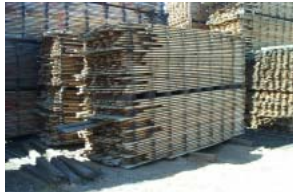
Figure7.41. Undesirable: Bearers out of line
