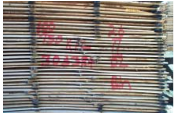
Figure 7.28. Undesirable: Poorly aligned rack sticks
