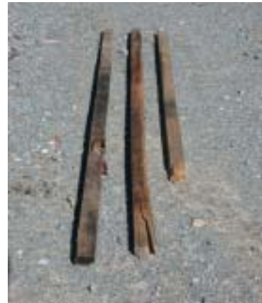
Figure 7.32. Rack sticks in poor condition discarded
