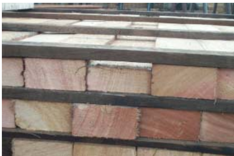
Figure 4.01. Result of poor cutting
