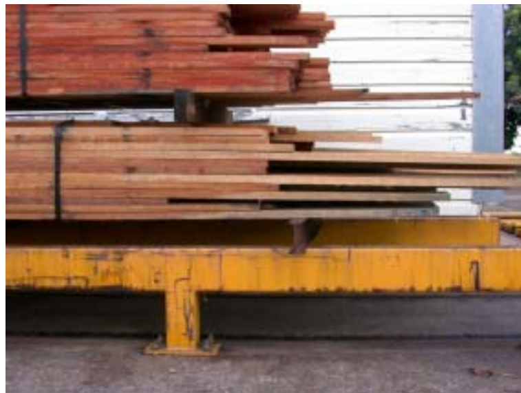
Figure 5.15. Unevenly built packs with unsupported board ends
