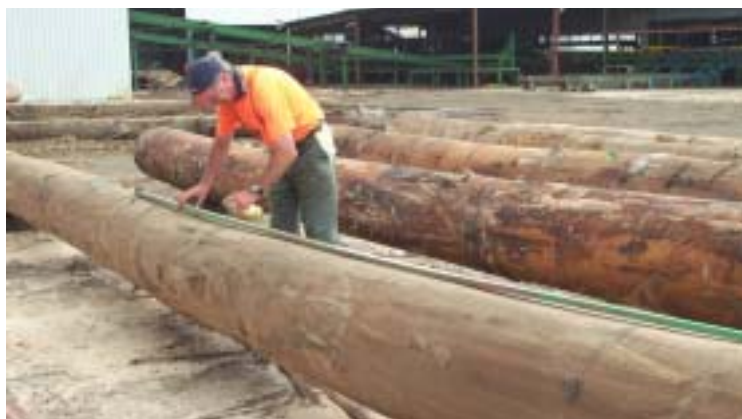
Figure 3.16. Measure the logs with a gauge
