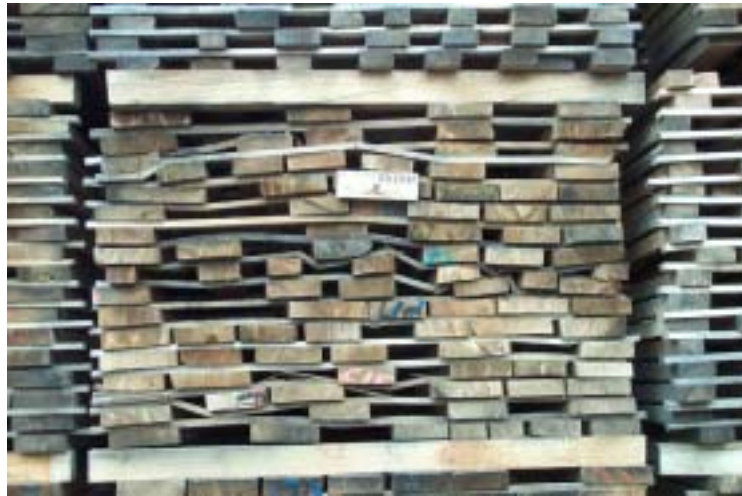
Figure 7.23. The results of poor racking practice
