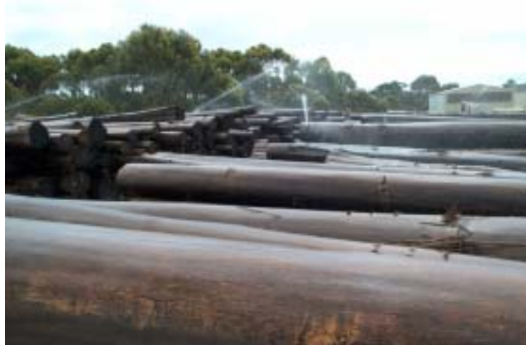
Figure 3.15. Sprinklers covering the logs well
