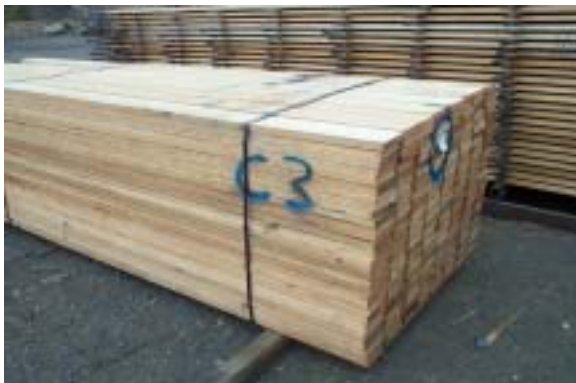
Figure 5.11. Desirable: Neat sides and ends
