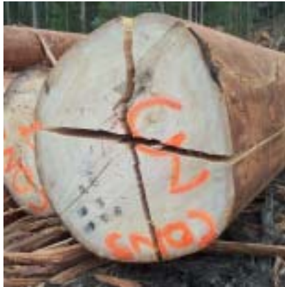
Figure 2.04. Log end splitting, caused by felling, initial drying, growth stress release or all three
