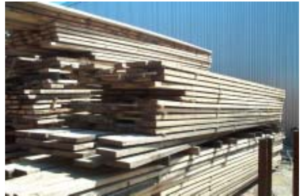
Figure 7.35. Undesirable: Uneven edges to a rack
