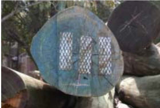
Figure 2.06. Metal and plastic end split restraints
