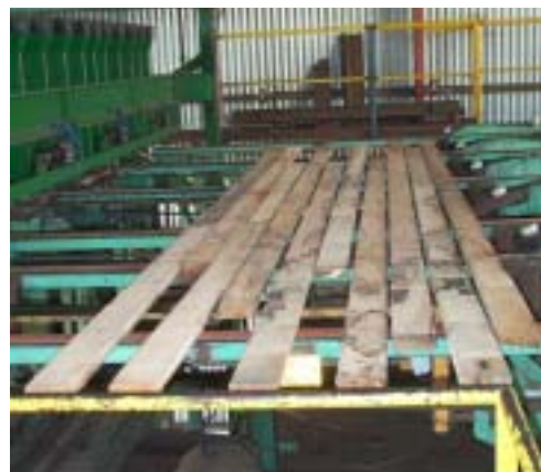
Figure 7.38. Top & tailing on a racking machine
