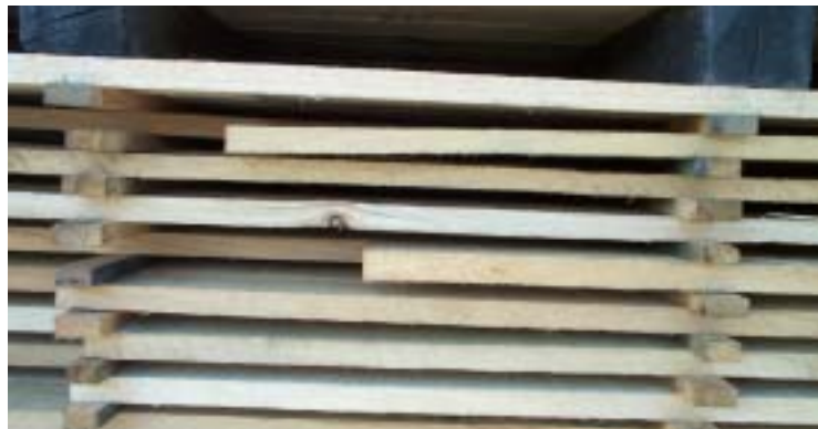
Figure7.43. Unsupported board ends distort during drying. This can be seen in the board second from the top
