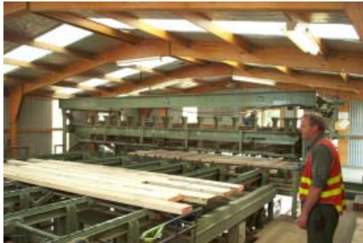
Figure 7.17. Boards are topped and tailed before being stacked mechanically
