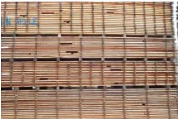
Figure 7.40. Desirable: Bearers and gluts in line
