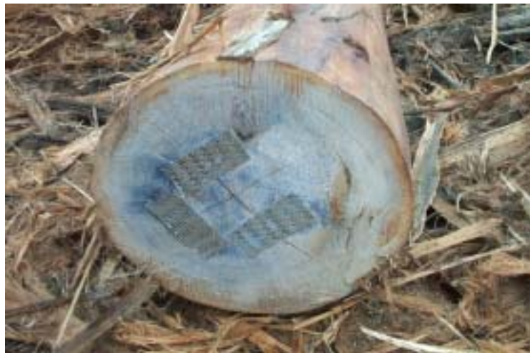
Figure 2.05. Metal nail plates used to restrain end splits
