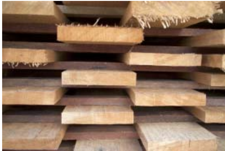
To distribute loads evenly throughout a stack, rack sticks should be placed directly one above the other in a vertical line. As the rack is assembled, when it is complete and when it is repositioned, the rack sticks should be straightened so that they remain in vertical lines.
