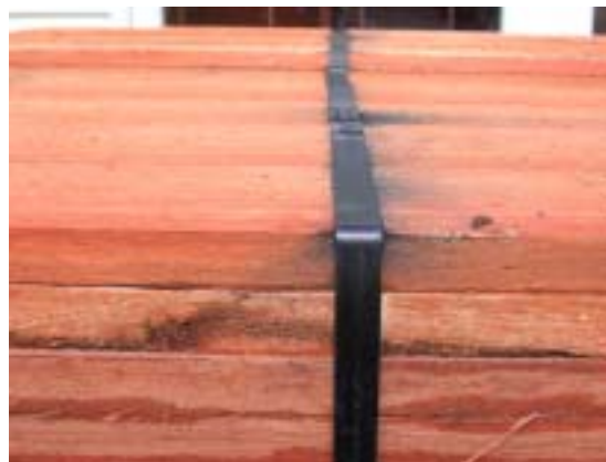
Figure 5.07. Undesirable: Corners crushed by pack straps
