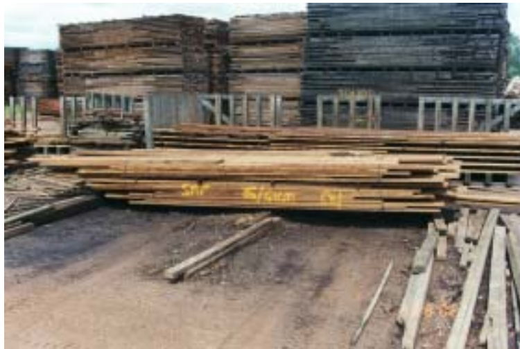
Figure 6.04 Packs in the sun can be damaged
