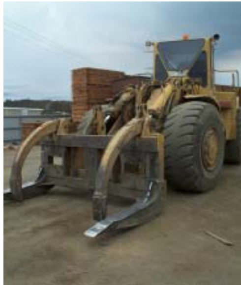
Figure 3.11. Heavy log loader
